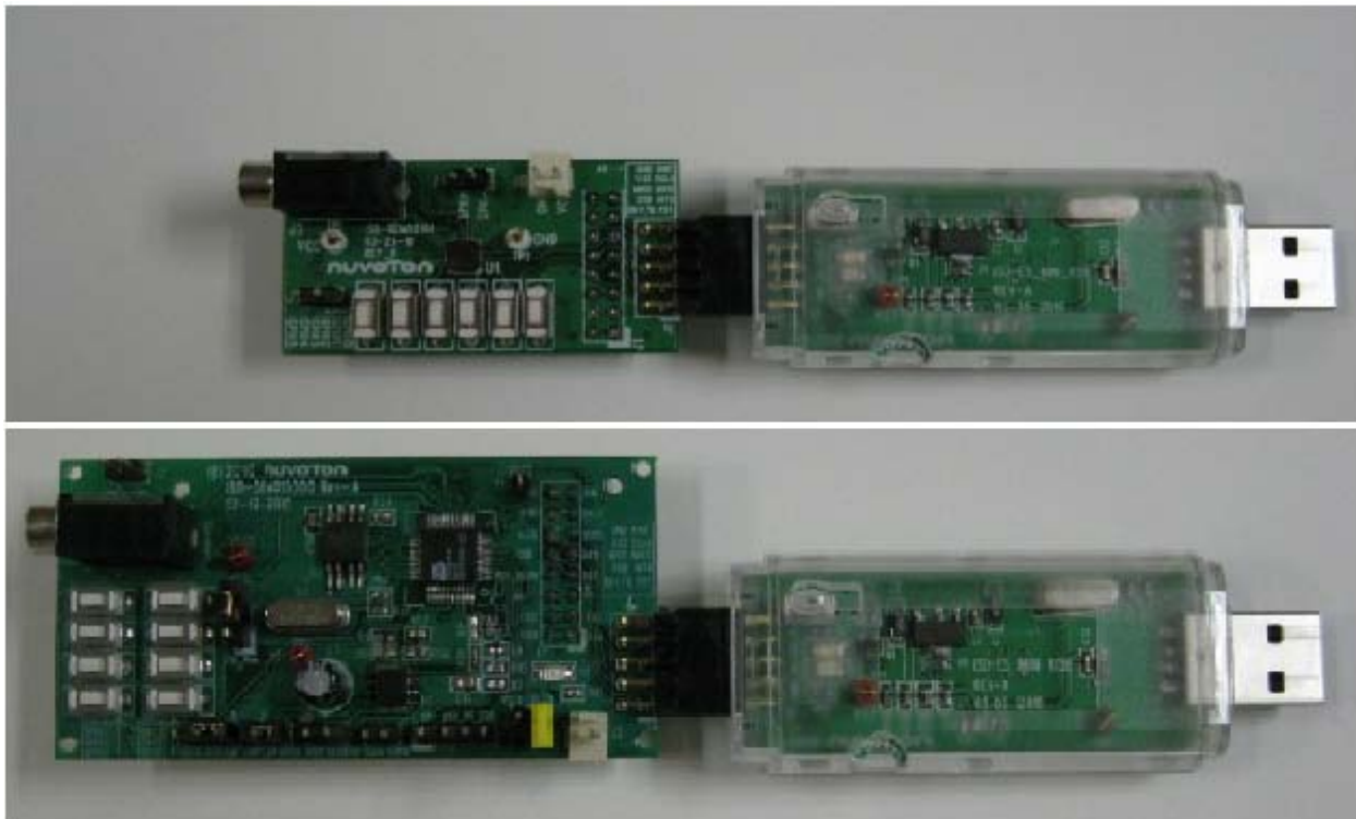
Figure 5 – To connect demo board and USB dongle: top side face up for both boards.
